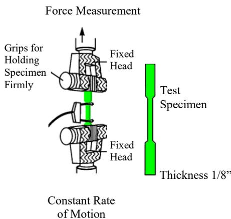
A piece of finished product, with a maximum thickness of .125-inches, is machined into a dog-bone shape. Each end of the test specimen is placed in opposite facing clamps which then attempt to pull it apart.
