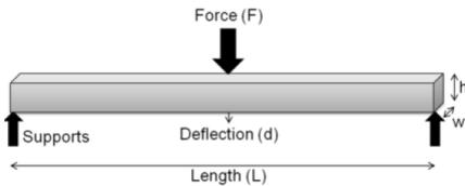
This test is used to measure the horizontal strength of the material. Supports are placed under the sample at each end, and then a piston drives down at the center. The force to drive down and the amount of deflection are measured to come up with the specimen’s **“Flexural Modulus”**.
